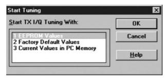
If user has PKD–1 dongle and other than NSM–X phone, then tuning is started automatically with EEPROM values. When using other dongles this selection opens same **Start Tuning** dialog as with TX Power Tuning.
