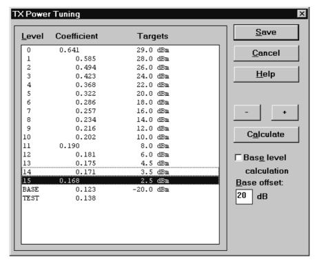
It is recommended that all the power levels are separately aligned although there is a possibility to align only three and calculate the rest. This is due to the calculation method.
